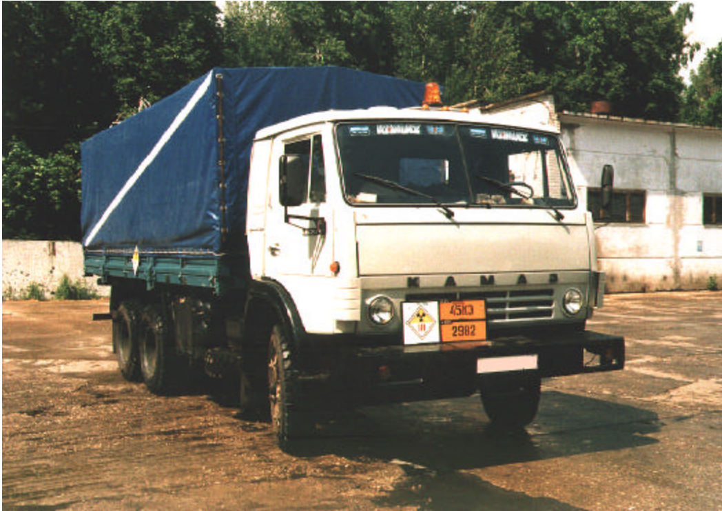
Figure 4, Special vehicle for transportation of radioactivity
