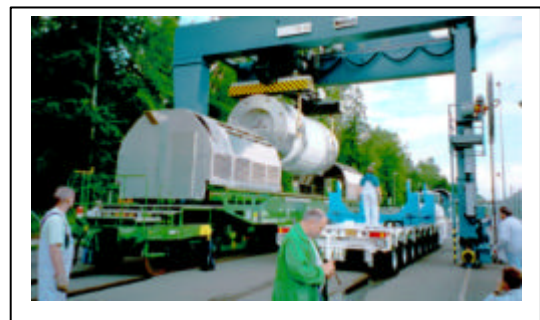
TN24 G tilting operation (Gösgen) and transfer by road to Zwiilag plants (Switzerland)
