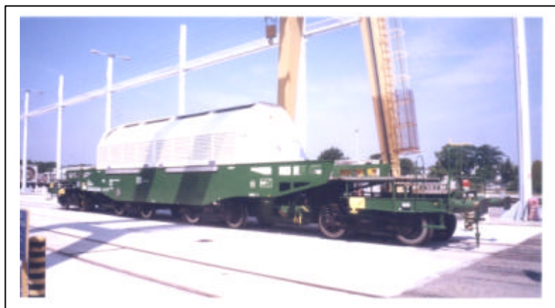
Fig. 1: Q76 rail wagon in transport condition
