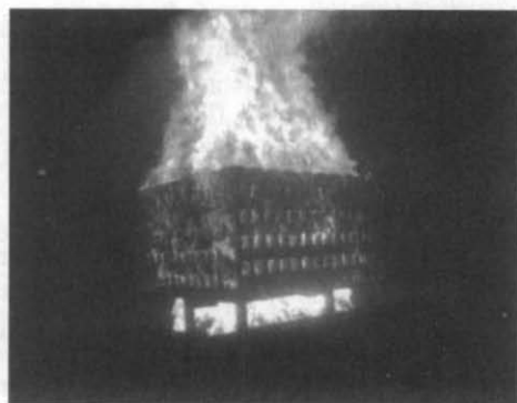
A simulated cargo fire test using a wood crib. This test was conducted in 1995 on the Mayo Lykes, a cargo freighter located at the U.S. Coast Guard test site in Mobile Bay, Alabama.
