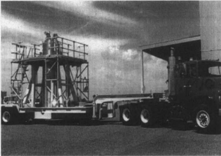
Figure 2 – Cask Transportation System
