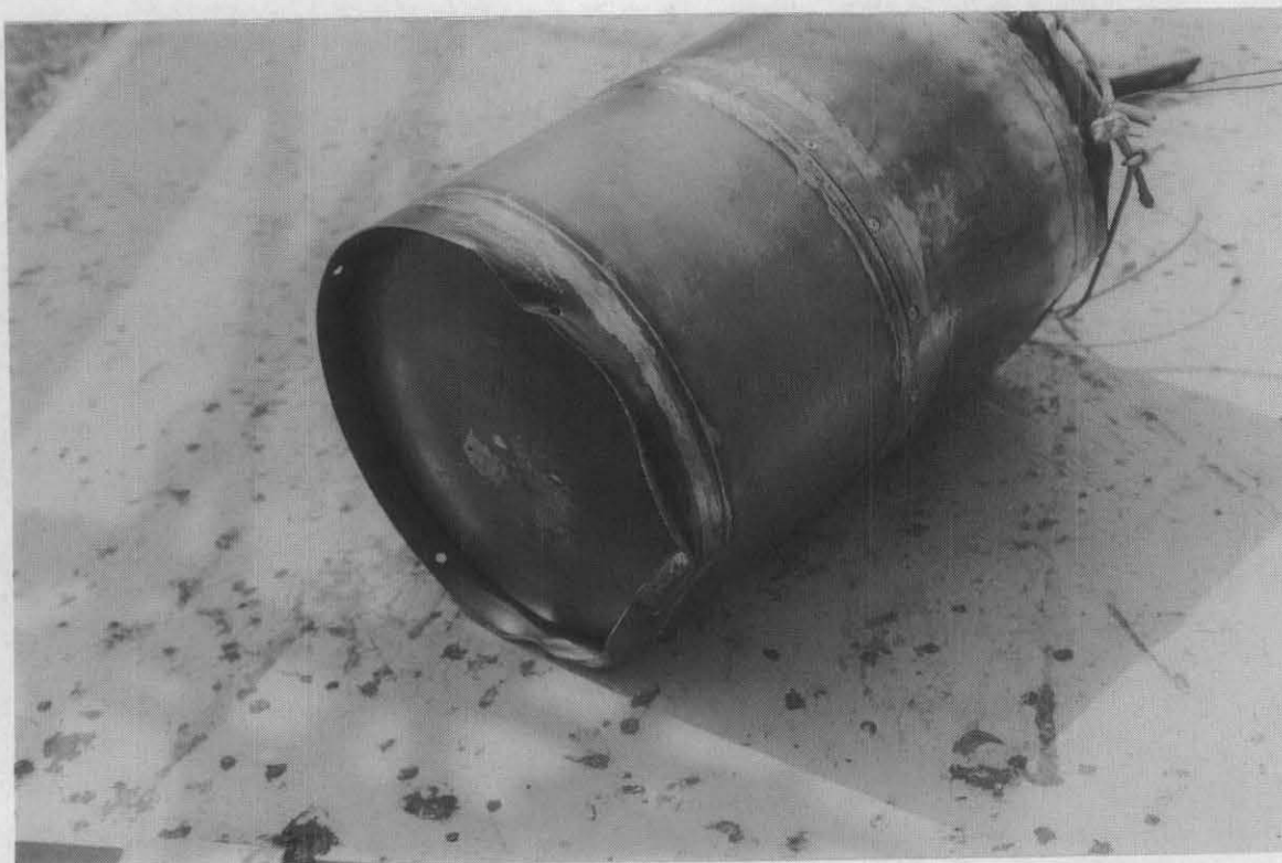
Fig. 5 - 1/2 Scale model deformation after 9m drop test
