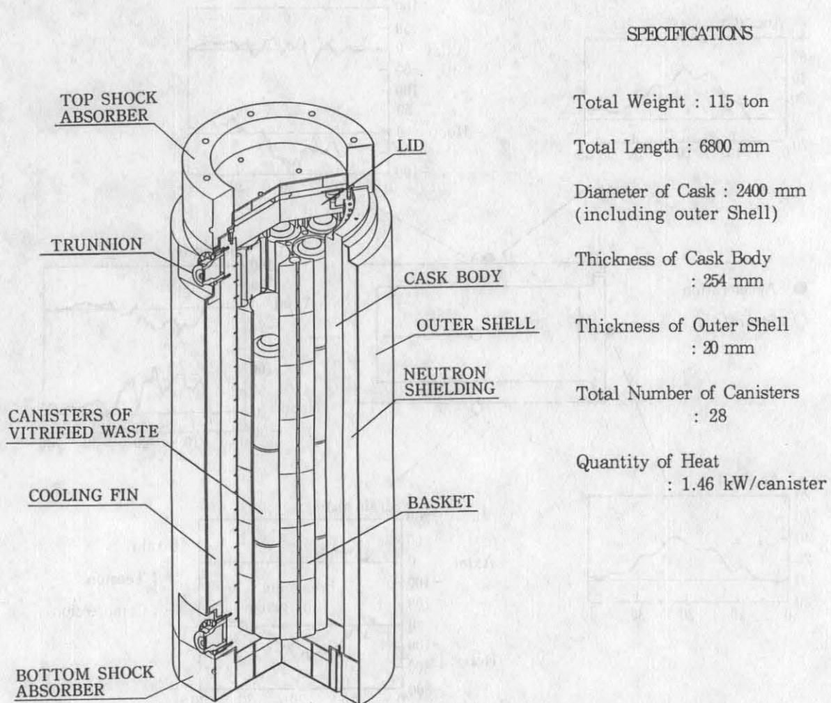
Fig. 1 Concept and Specifications of Demonstration Test Cask
