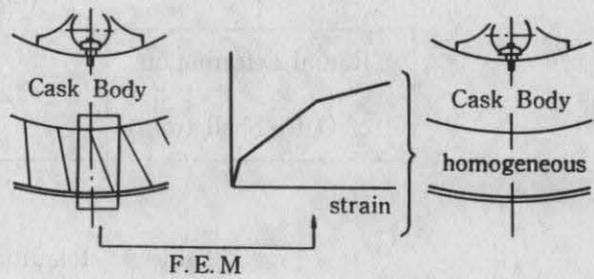
Fig. 5 Procedure for Obtaining Stress-Strain Curve of Neutron Absorber
