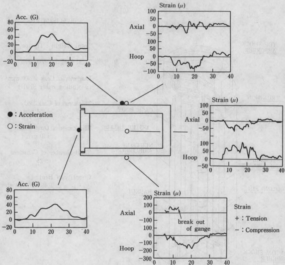
Fig. 2 Acceleration and Strain Time Histories
