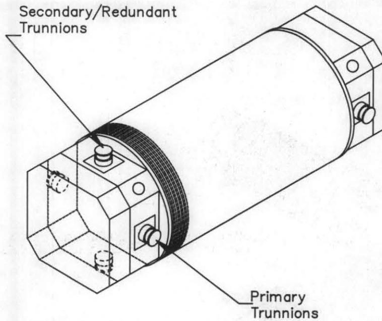
FIGURE 3 - CASK HAVING PRIMARY AND SECONDARY/ REDUNDANT TRUNNIONS
