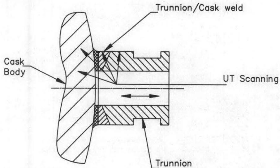
FIGURE 4 - EXAMPLE OF UT TESTING OF TRUNNION/ CASK WELD
