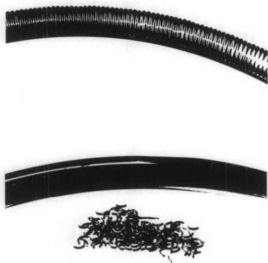
Fig. 8. Top: X-ray radiograph of a HELICOFLEX gasket with Al-lining after 40,000 load cycles ( 10 \text{ kN} \leq F \leq 75 \text{ kN} ) Bottom: Destruction of the spring core
