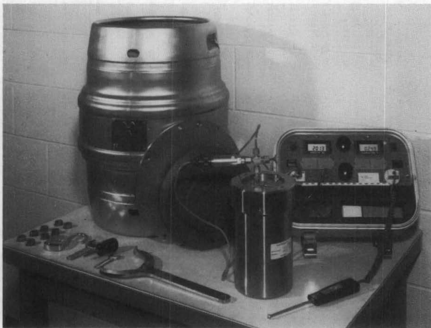
FIG. 1. SAFKEG package design No. 2799E with the containment vessel being leak tested using a CALT pressure drop leak tester.
