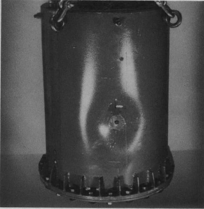
FIG. 8. Mantle deformation of a 1:3 model after the 1 m drop.
