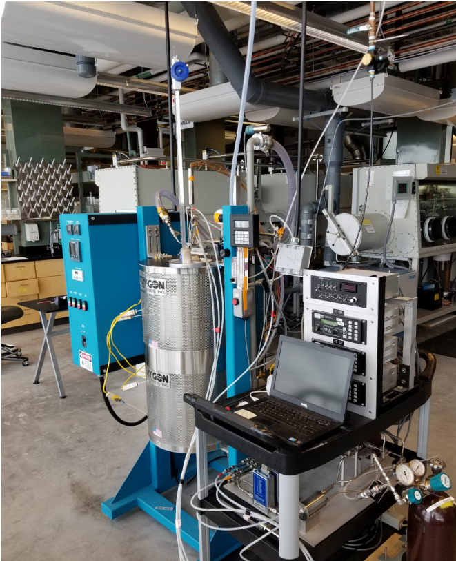
Figure 2. Photo of the two-zone furnace including the bubbler control panel.
