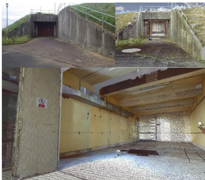
**Figure 2.** Complex data to complex form: terrestrial laser scanning data. **Top left:** Photograph of the entrance of one of the bunkers used during LETTERPRESS. **Top right:** Laser scan data from the same bunker displayed in GeoVisionary and replicating the photograph. **Bottom:** View from inside that bunker.
