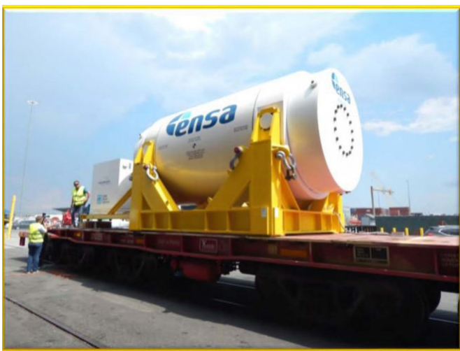
Figure 2. Railroad Transport Mode of the Test Cask in the United States
