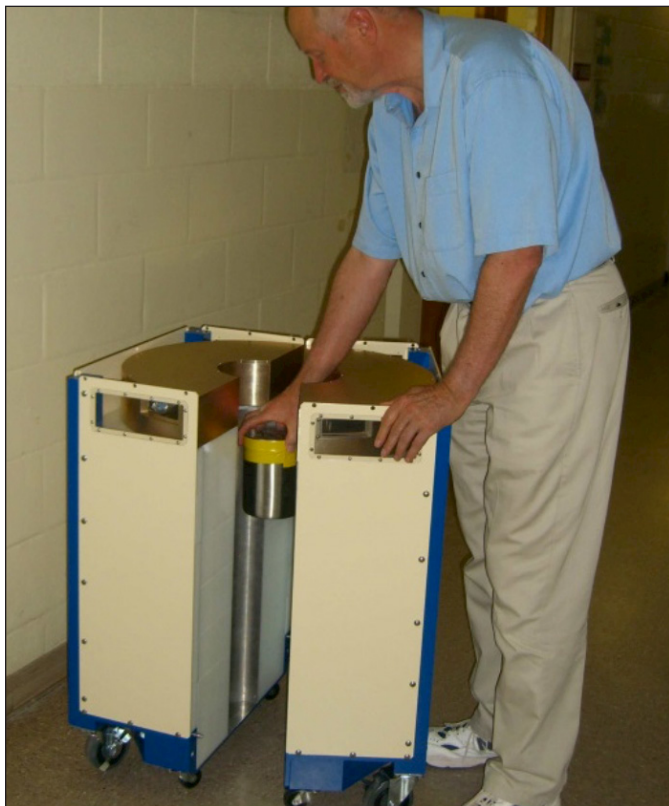
Figure 15. The high efficiency mini-ENMC with split geometry for inserting plutonium samples or FBR assemblies
