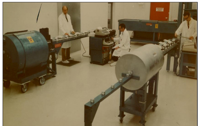
Figure 1. Two NDA systems used at the Hanford, FFTF fabrication plant in 1972 to measure the plutonium mass and isotopic ratios for the MOX fuel rods. The left system is a ^{252}\text{Cf} active/passive gamma scanner for pellet measurements, and the right system is a neutron coincidence system for the ^{240}\text{Pu}_{\text{eff}} mass. 3
