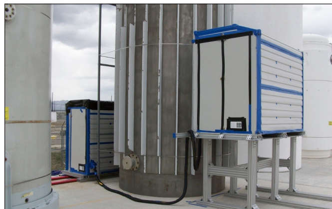
Figure 3. Muon tracking detectors in weatherproof enclosures around the MC-10 cask at Idaho National Laboratory. One detector is elevated relative to the other to take advantage of the higher muon flux at smaller zenith angles.
