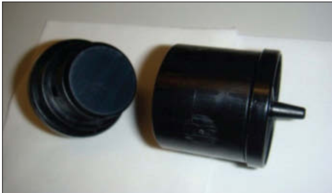
Figure 2. Deposition of particles using an inertial impactor for LG-SIMS samples at IAEA
