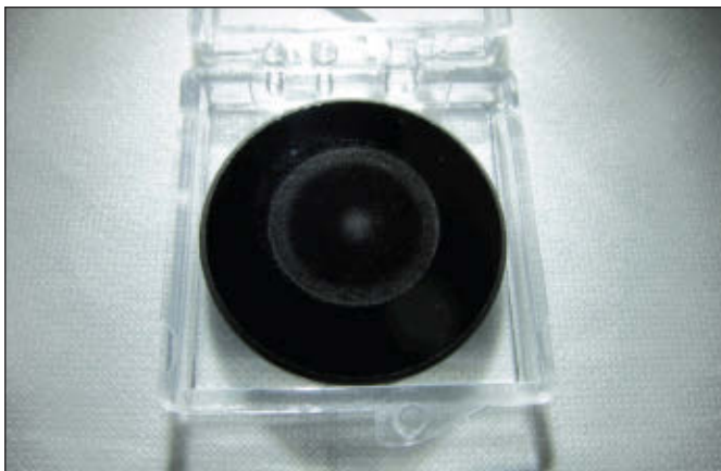
Figure 2. Deposition of particles using an inertial impactor for LG-SIMS samples at IAEA
