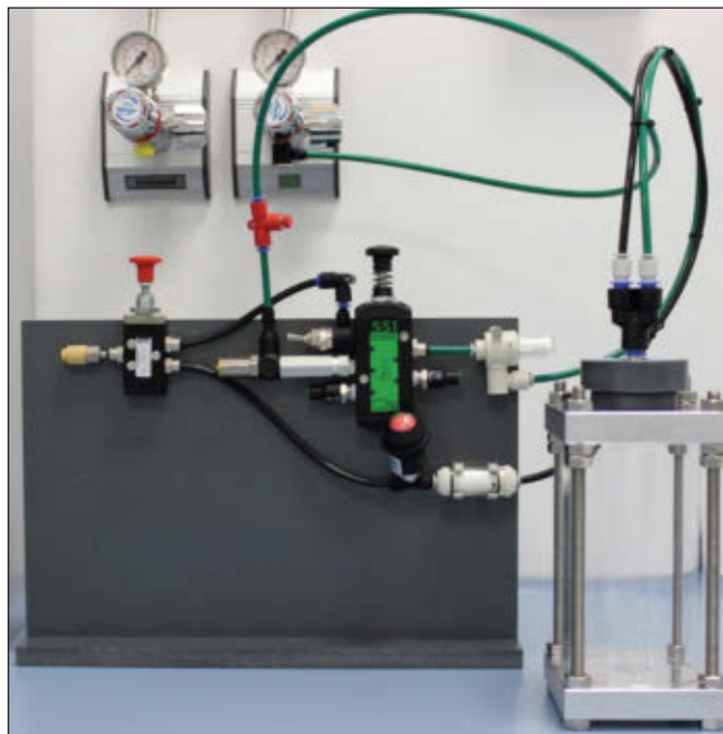
Figure 6. Prototype of shock wave disperser device
