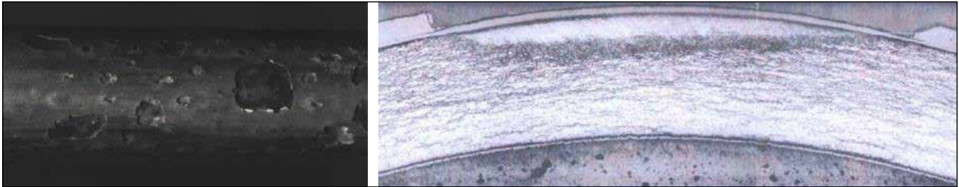
Figure 4. Oxide layer spalled from the fuel cladding surface material
