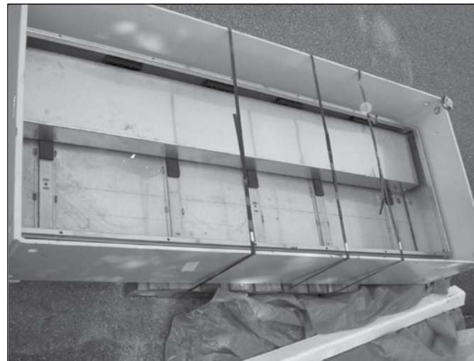
Figure 11. The completed NDM, installed in its stainless steel envelope, can be seen in place inside the open NEMA 4 enclosure, which is inside of the steel shroud.
