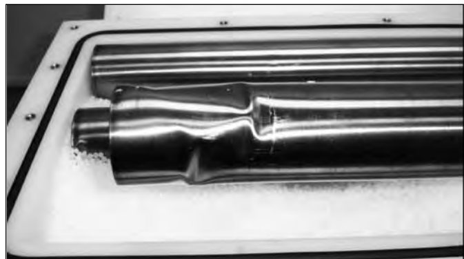
Figure 8. A close-up view of the most damaged tube from the drop test mock-up. While wrinkled, the tube has not been breached. The tube is being held above its installed position in the mockup for this photo.
