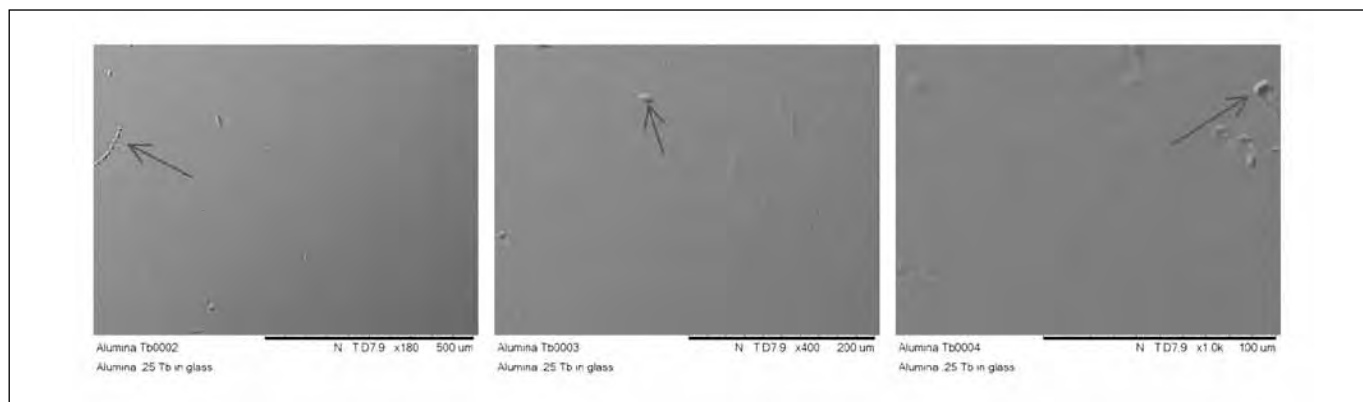
Figure 5. SEM micrograph (topography mode acc V-15 keV wd-7.9) of synthesized alumina gel deposited in corning glass surface by spin coating methods (400 rpm, 15 sec). Magnification from left to right 180X, 400X and 1000X.
