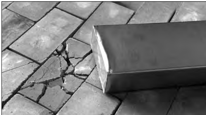
Figure 5. This is a side view of the assembly after impact, showing deformation of the case.
