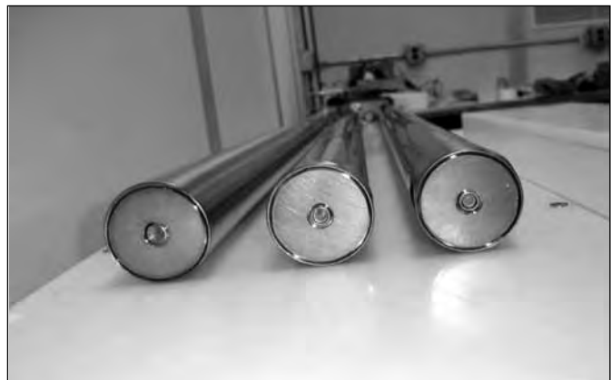
Figure 8. A close-up view of the most damaged tube from the drop test mock-up. While wrinkled, the tube has not been breached. The tube is being held above its installed position in the mockup for this photo.
