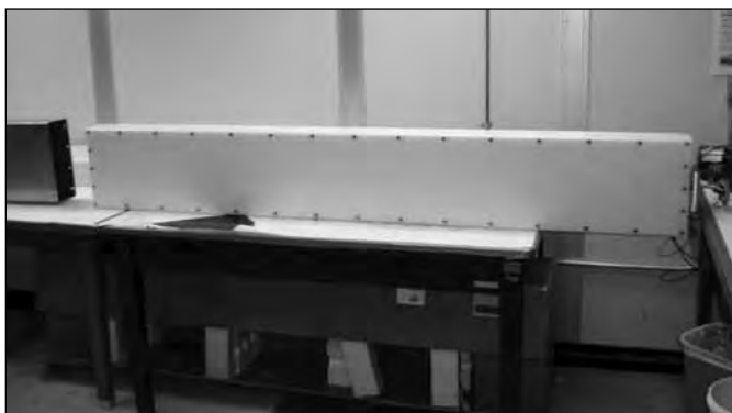
Figure 6. The polyethylene cavity after being slid out of the stainless steel envelope
