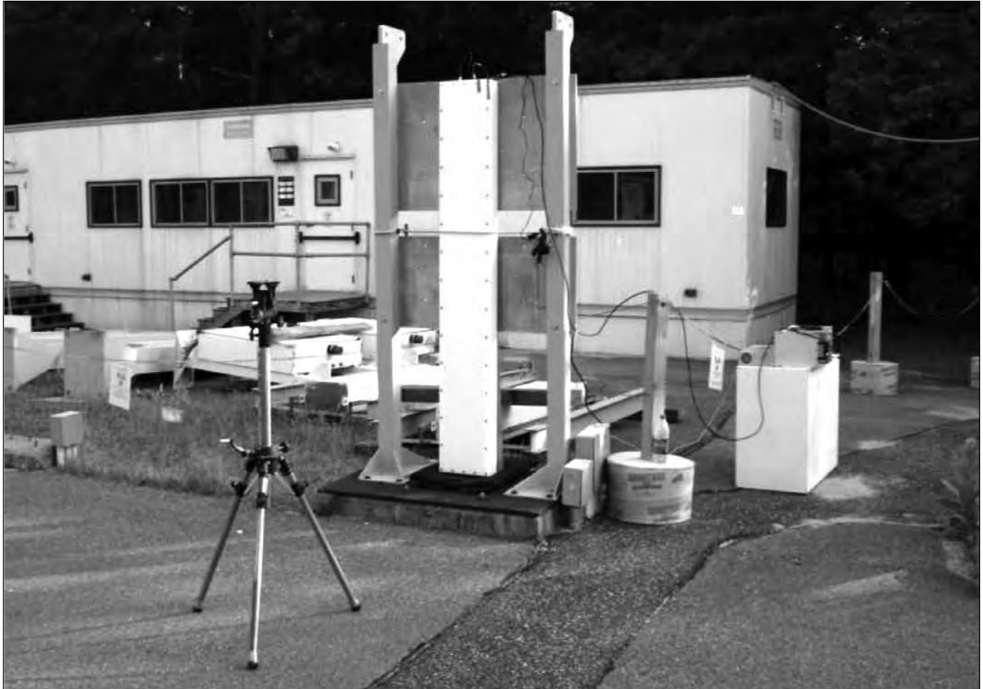
Figure 9. The detector module is seen here mounted on a footing at the former RADTEC site, for sensitivity tests.
