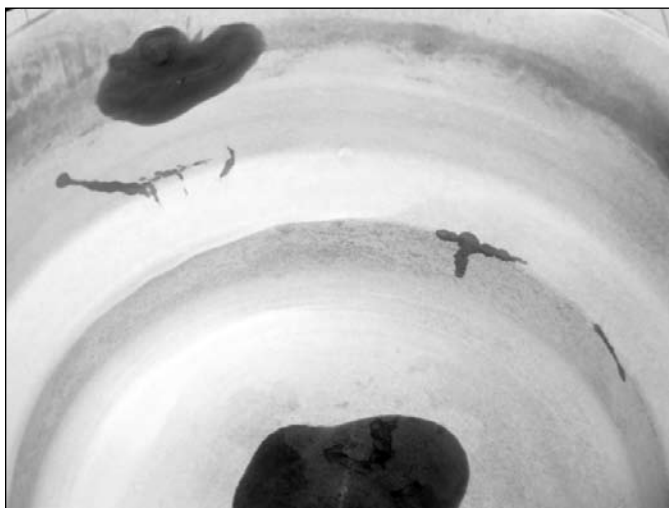
Figure 7. Dye penetrant testing of 3013 inner container bottom section; dark lines indicate crack locations and dark spots are the drilled hole locations
