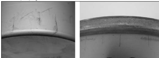
Figure 12. Stress-corrosion cracks in 3013 container sections exposed to boiling MgCl_2 Solutions
