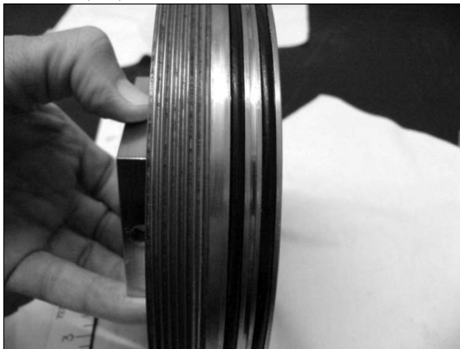
Figure 4. O-ring seal from 9975 shipping package primary containment vessel (PCV)
