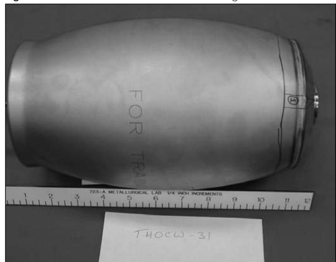
Figure 7. 3013 outer container after burst testing
