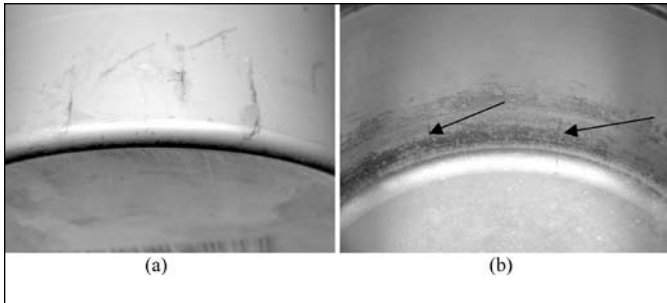
Figure 4. Metallographic cross section of through-wall crack at the container to base fabrication weld in 3013 outer container after boiling magnesium chloride test: a) Overall macrograph showing base of container through fabrication weld and container body; b) Stress-corrosion crack from sample shown in (a). Note the crack branching and the position of the crack, beginning in the weld region and propagating into the base of the container
