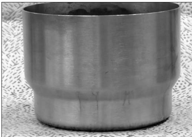
Figure 11. Convenience container section after exposure to boiling magnesium chloride solution: container exterior with axial cracks in sidewall
