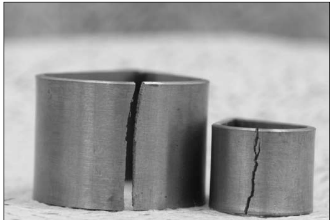
Figure 12. 304L teardrop coupons after exposure to a boiling magnesium chloride solution
