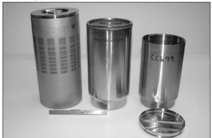
Figure 1. The 3013 container used by Savannah River Site (SRS) for oxides. The outer container is consistent for all packaging sites in the DOE Complex.
