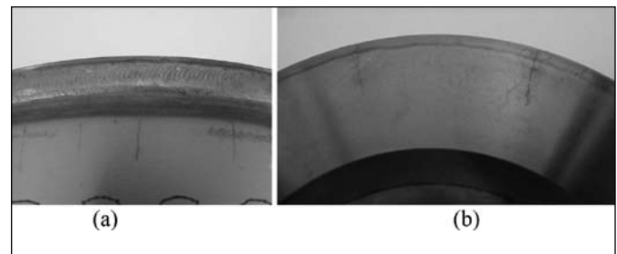
Figure 5. Top half of GTAW closure welded 3013 outer container section with through-wall cracks after boiling magnesium chloride test: a) Exterior of container with cracks perpendicular to GTAW weld and running into container body (b) Exterior of lid showing appearance of cracks perpendicular to GTAW weld in lid
