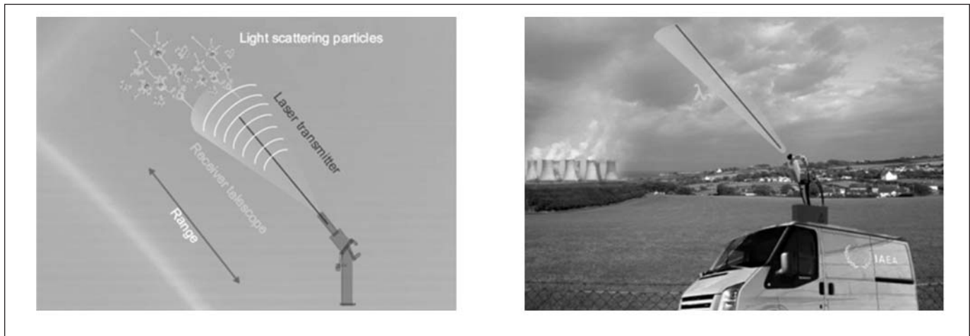
Figure 8. Left: A simplified diagram explaining the laser-based stand-off detection method Right: An artist impression of a mobile laser-based stand-off detection unit
