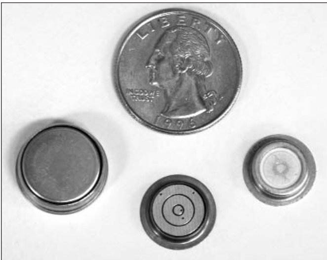
Figure 1. Examples of three commercial contact memory buttons, with a U.S. quarter shown alongside for scale
