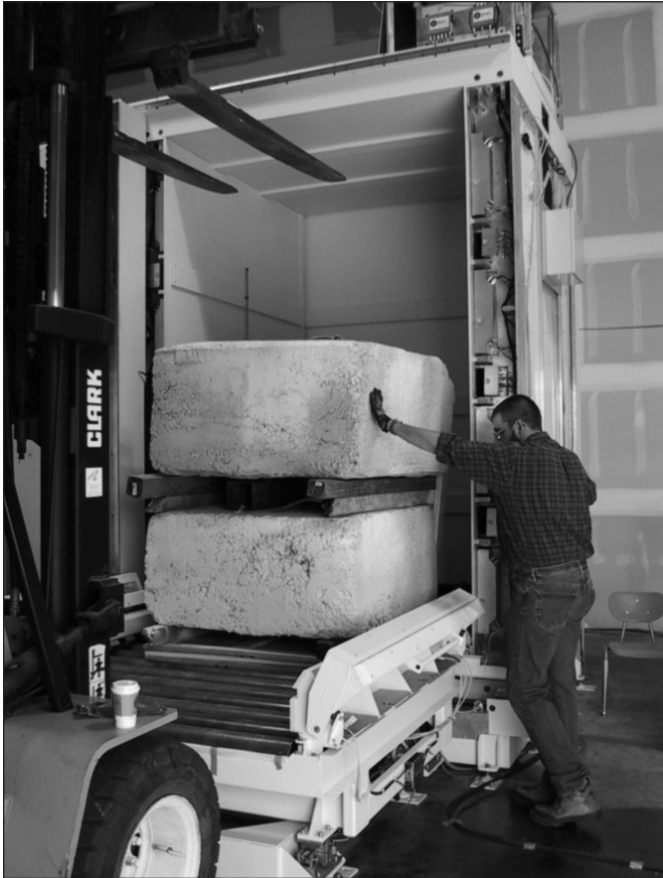
Figure 15. WCAS-B concrete block load testing in Albuquerque, New Mexico, in October 2001. The WCAS-B is now used in the Rokkasho Reprocessing Plant in Japan.
