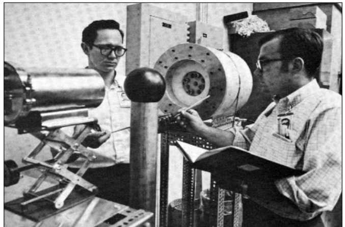
Figure 2. TA-18 Fast-neutron interrogation. Henry and Masters performing active assay of a uranium sphere using prompt and delayed neutrons in 1969
