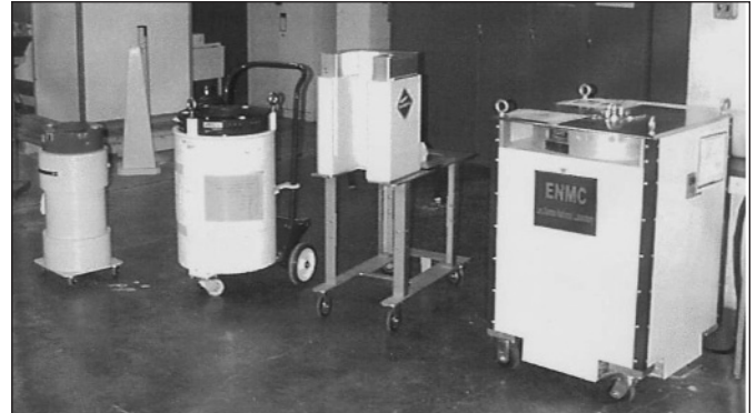
Figure 24. AMPTEK and 3 He-tube-based neutron-based NDA family
