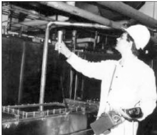
Figure 4. GGH applied in a uranium facility to measure an overhead duct
