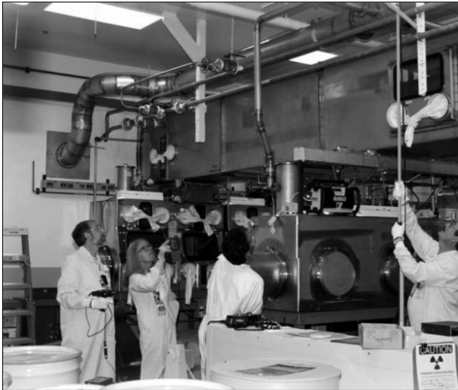
Figure 5. A compact NaI detector is shown during measurements of plutonium deposits in overhead ducts.
