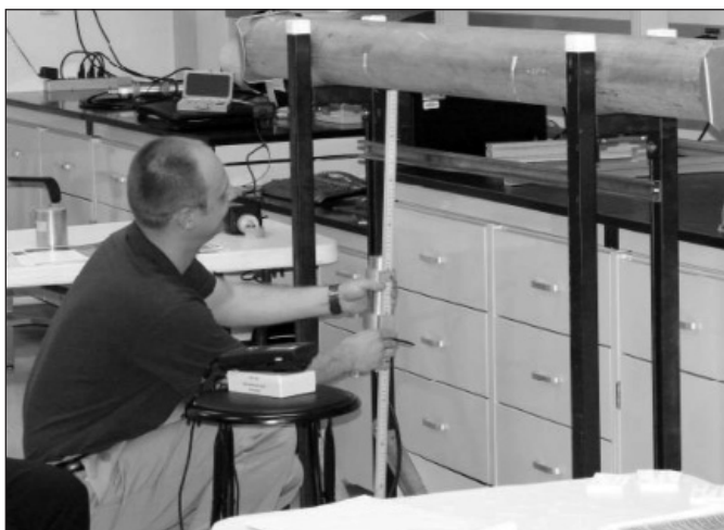
Figure 9. Alexander Solodov (ORNL) prepares to make a holdup measurement on a small round duct.
