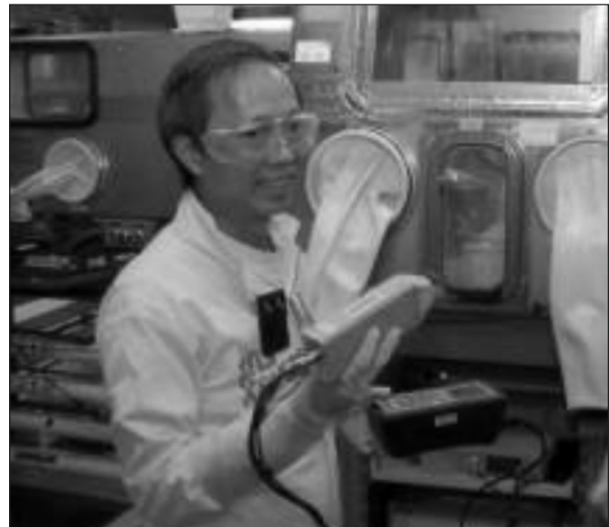
Figure 2. The Peltier-cooled CdTe detector is shown measuring Pu isotopic composition in a glovebox.
