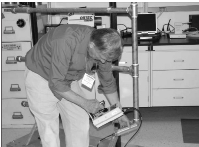
Figure 9. Alexander Solodov (ORNL) prepares to make a holdup measurement on a small round duct.
