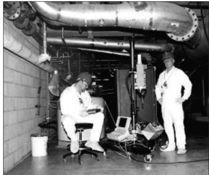
Figure 7. Measurements of 235 U deposits in a filter system performed with CZT and NaI
