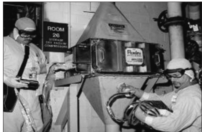
Figure 7. Measurements of 235 U deposits in a filter system performed with CZT and NaI
