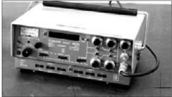
Figure 2. The Eberline SAM-2 electronics module with digital rate multiplier used for low resolution gamma-ray measurements and neutron totals counting
