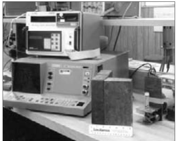
Figure 5. Silena Cicero MCA with LLNL's "Blue Box" plutonium isotopic analyzer. This was the first true Pu isotopic analysis system used by the IAEA.
