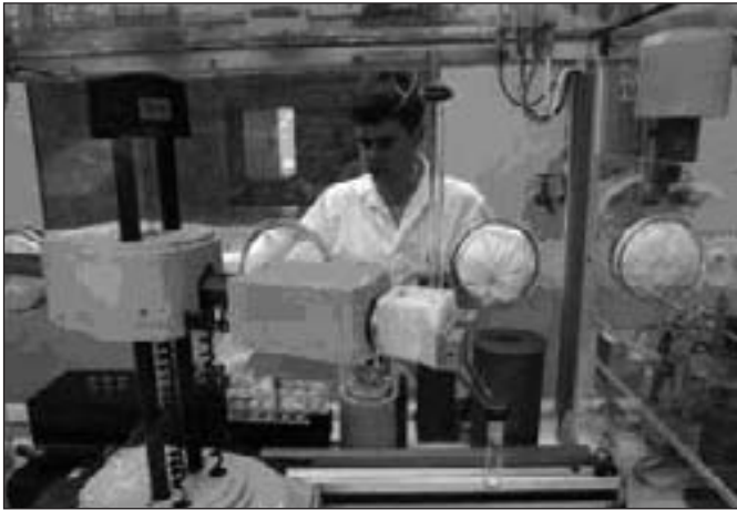
Figure 2: ITU chemical separation robot installed in a glove box
