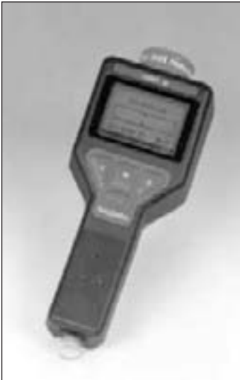
Figure 3. The handheld monitor HM-5 used for safeguards (method H and active fuel length) and illicit trafficking measurements
