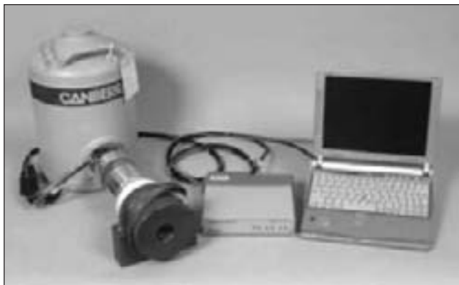
Figure 6b. InSpector-2000(IMCA) and Mini-Multichannel Analyzer (MMCA) are now the preferred gamma-ray instruments at the IAEA.
