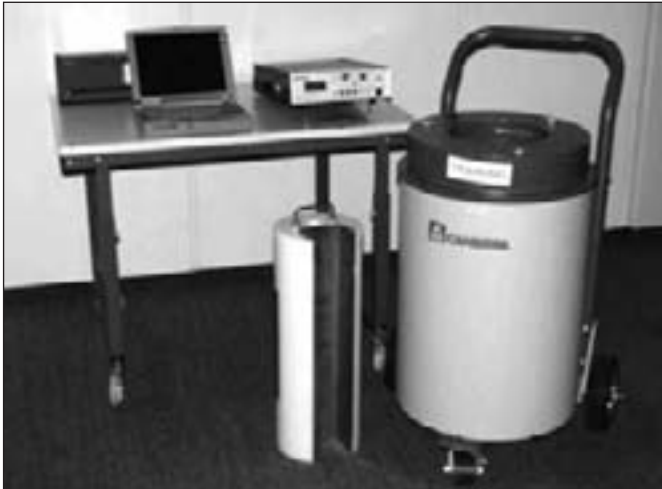
Figure 8. The AWCC with the MTR fuel element insert and JSR-12 electronics used for the verification of ^{235}\text{U} in bulk samples and MTR fuel assemblies
