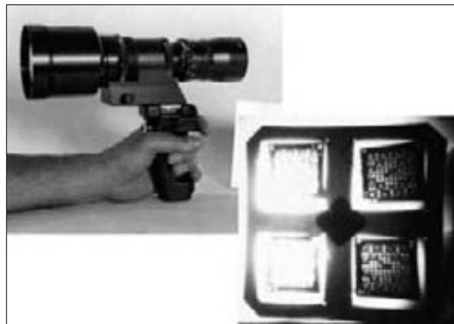
Figure 15. The original version of the CVD for the verification of the Cerenkov glow from spent fuel assemblies, more advanced versions of the CVD have been developed in recent years.
