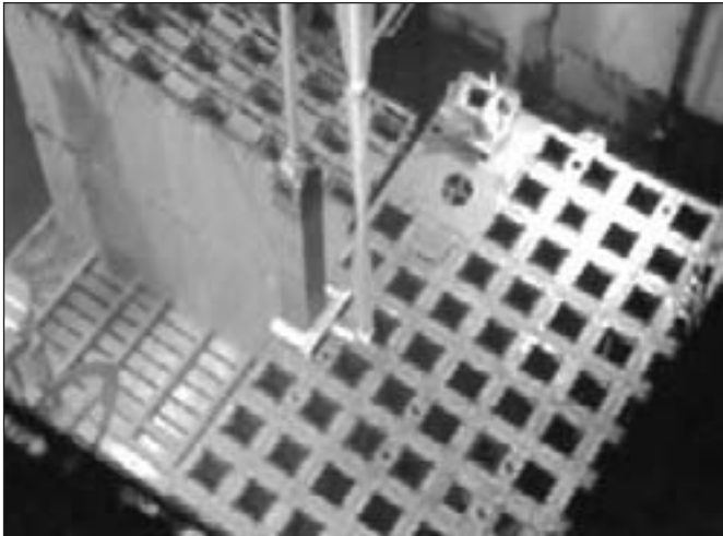
Figure 16. Underwater view of the Fork (FEDT) measuring the gross neutron and gamma activity from spent PWR fuel assemblies.
