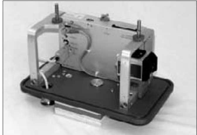
Figure 9. Single camera unit consisting of DCM14 data module and CCD-camera, Courtesy: Dr. Neumann Consultants
