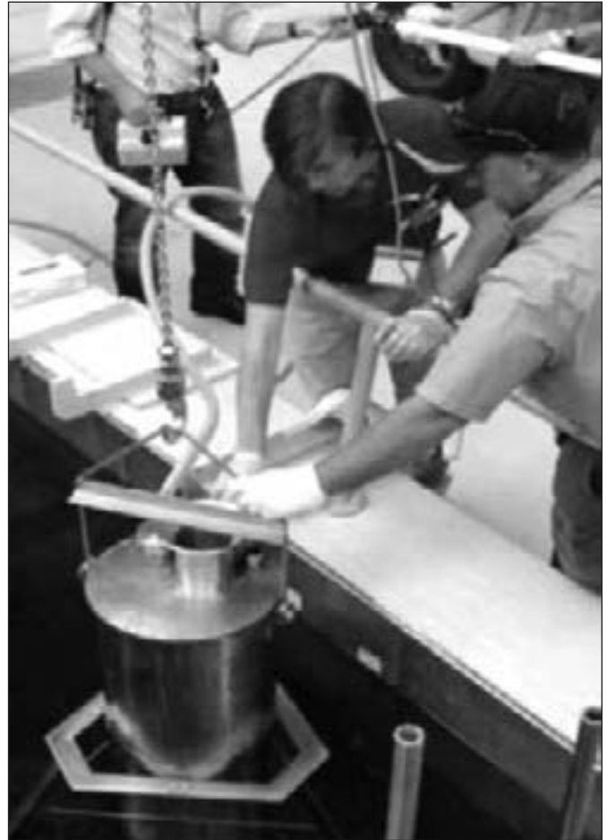
Figure 17. Alain Lebrun putting the AEFC into the spent fuel pool at the HIFAR reactor in Australia for an inspection verification of the spent fuel elements
