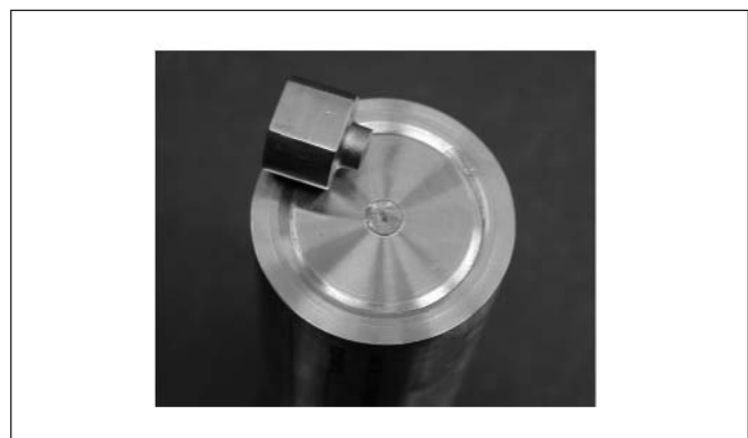
Figure 3. When the source is placed inside the capsule, the knob is sheared-off.
