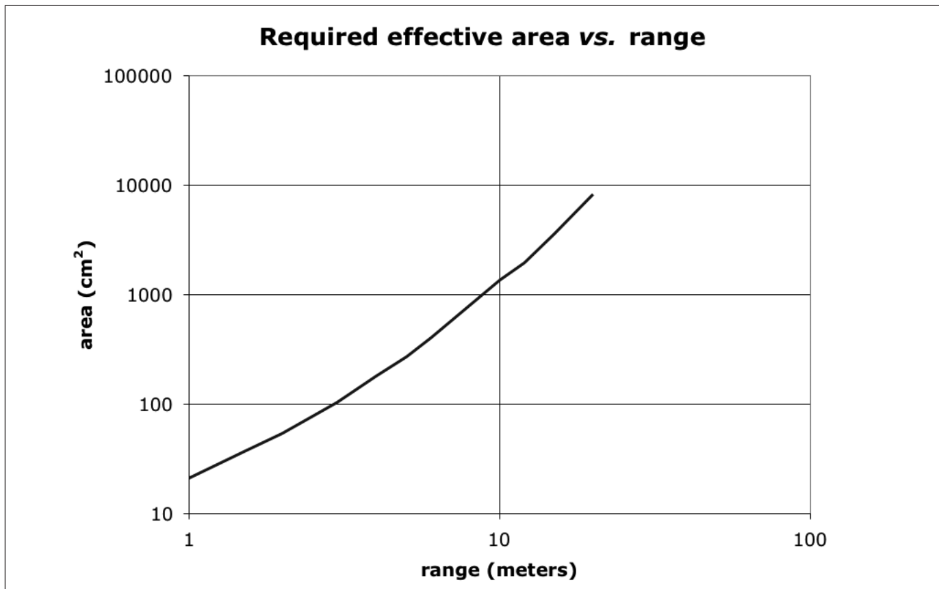
Figure 5. Size of a screening detector to detect a 7 \times 10^5 \text{ gamma s}^{-1} source moving past at 30 mph ( 13.4 \text{ m s}^{-1} ). This detector is the first in a two-step detection strategy, and is followed by a much smaller mobile detector to confirm the detection with high confidence.
