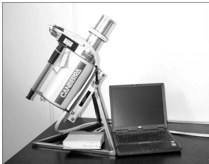
Figure 1. Detector system (detector, MCA, computer, NATE and absorber plate) during analysis of a U_3O_8 standard for calibration
