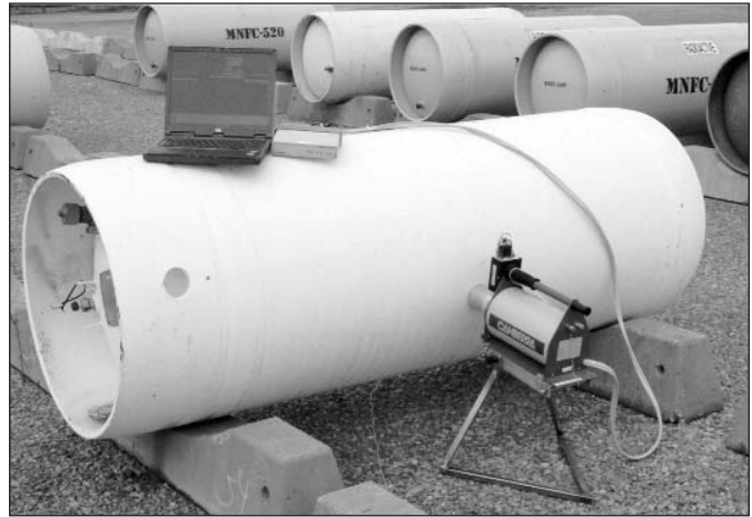
Figure 2. Detector system set up on the side of a type 30B LEUF 6 cylinder
