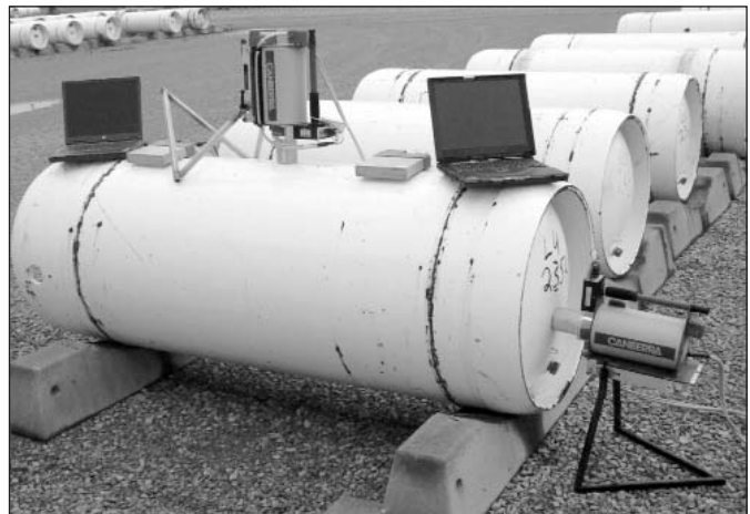
Figure 3. Two-detector system set up at top and end locations of a type 30B LEUF 6 cylinder
