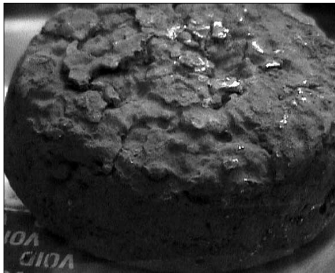
Figure 3. A 2-kg Pu metal button upon removal from SRS bagless transfer can
