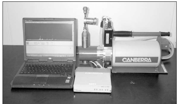
Figure 3: Measurement system including the LEGe detector, MCA, computer, and sample cylinder. The sample cylinder is held in place with the ALEX attachment ensuring geometrical reproducibility.
