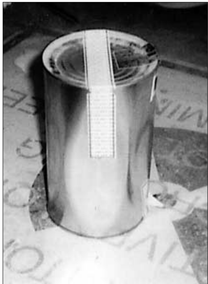
Figure 4. Photograph of a paneled rim-sealed Hanford container of plutonium metal that did not release contamination. Several examples of the paneling phenomenon are listed in Table 3.
