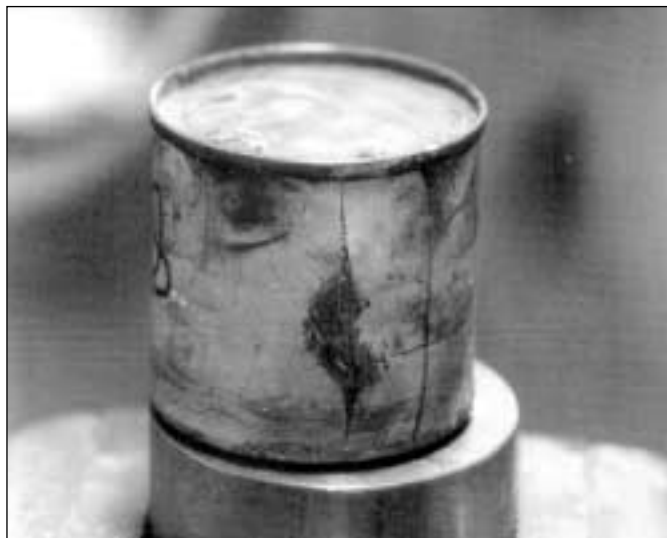
Figure 1. Photograph of a rim-sealed aluminum container that ruptured due to excessive mechanical pressure from oxidized plutonium metal, due to a faulty seal. This event occurred at Rocky Flats in 1982 and is described as case Seal-4 in Table 1.
