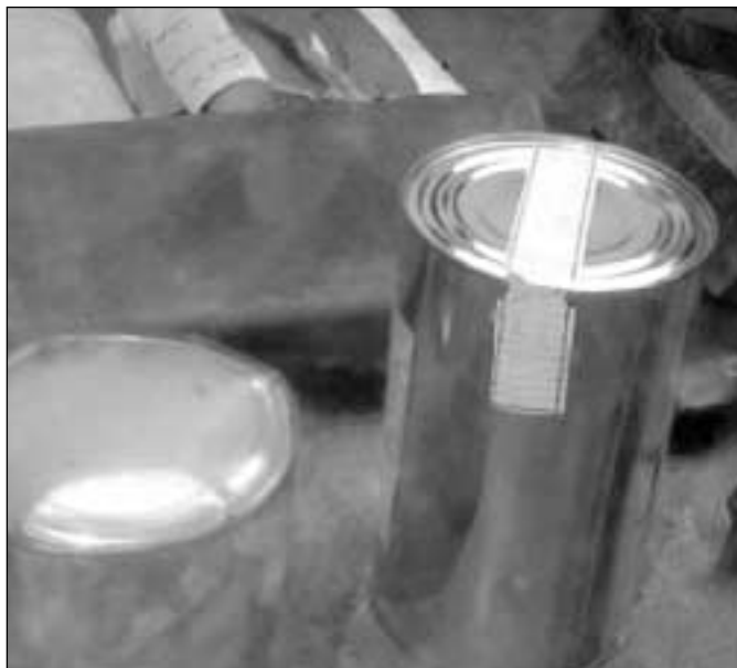
Figure 5. Photograph of a bulged Hanford rim-sealed container of plutonium oxide that did not release contamination. Other examples of the bulged can phenomenon are given in Table 3.
