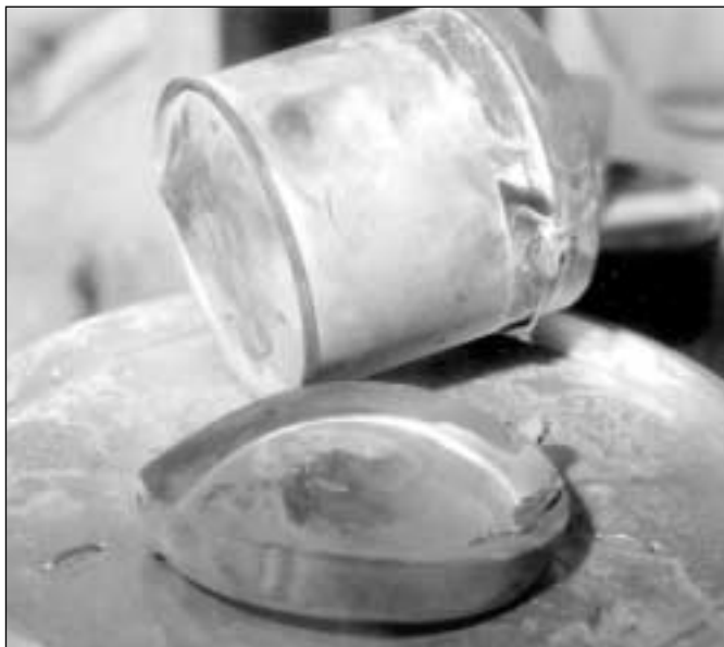
Figure 3. Photograph of a slip-lid can that ruptured due to excessive gas pressure. This event occurred at Hanford in 1980 and is described as case Pressure-5 in Table 2.
