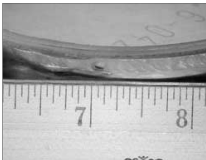
Figure 2. Photograph of a defective closure weld on a stainless-steel storage container that led to an incident in September 1999 at Savannah River; causing intake of plutonium by seven workers and extensive vault contamination. This event is described as case Seal-9 in Table 1.
