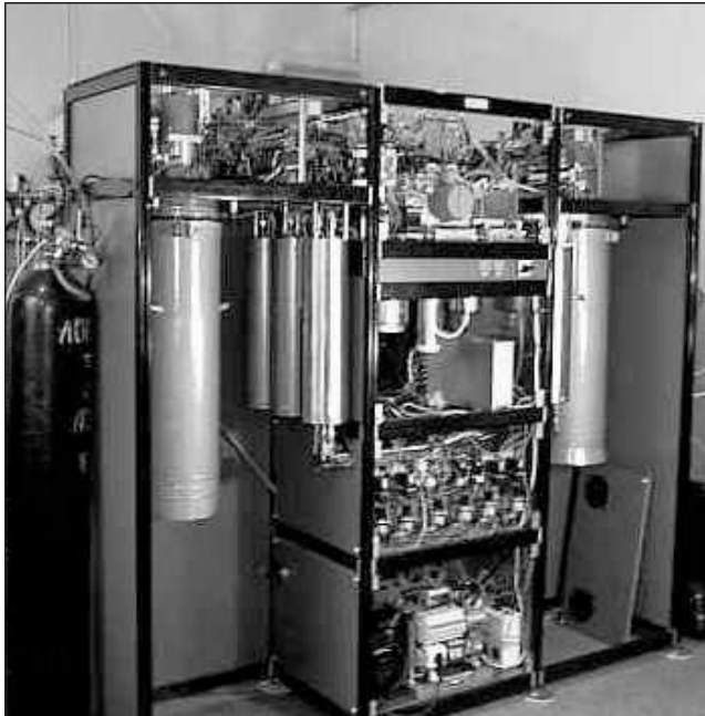
Figure 2a. Noble gas system Arix (KRI, Russia)
