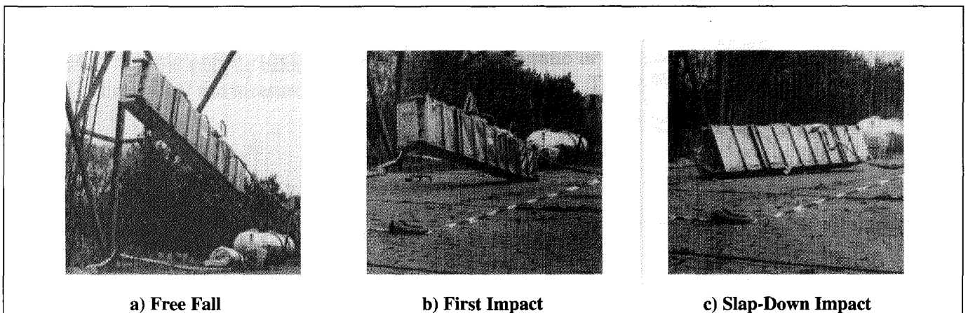
Figure 11. ANF-18. 9m and 15° declined drop test
