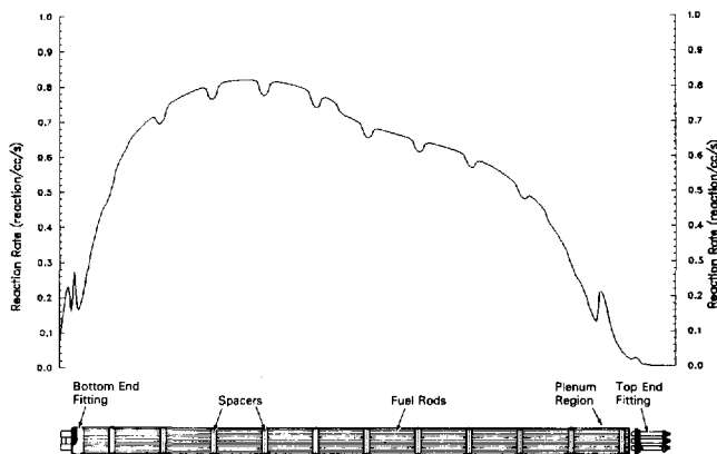
Figure 2. Co-59 (n,gamma) Normalized Reaction Rate for a Combustion Engineering Fuel Assembly
