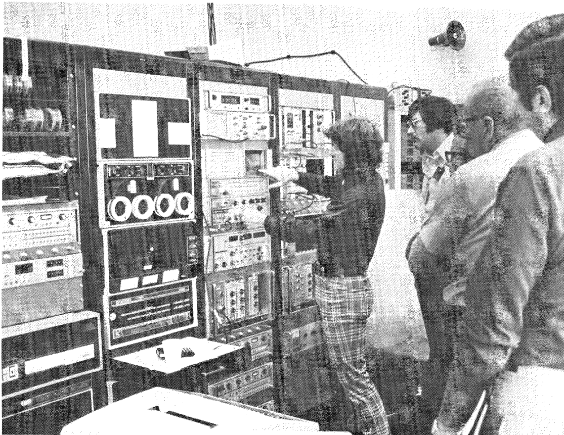
Figure 7. LASL instructor, D. Reilly, demonstrates operation of a segmented gamma scan (SGS) system. The pictured system is a versatile data acquisition system for laboratory use. Dedicated SGS systems are much smaller and simpler to operate.
