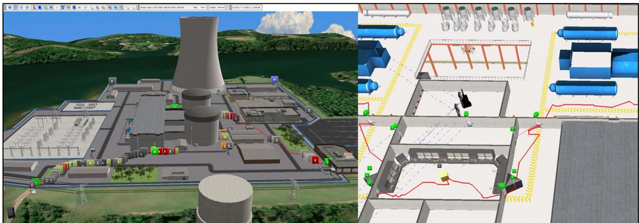
Figure 1. AVERT-PS 3D Digital Twin model of a hypothetical nuclear power plant, site and interior details.
