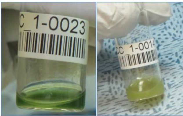
Picture 1. Example of successful dissolution (left) and sample that exhibited dissolution difficulties (right).
