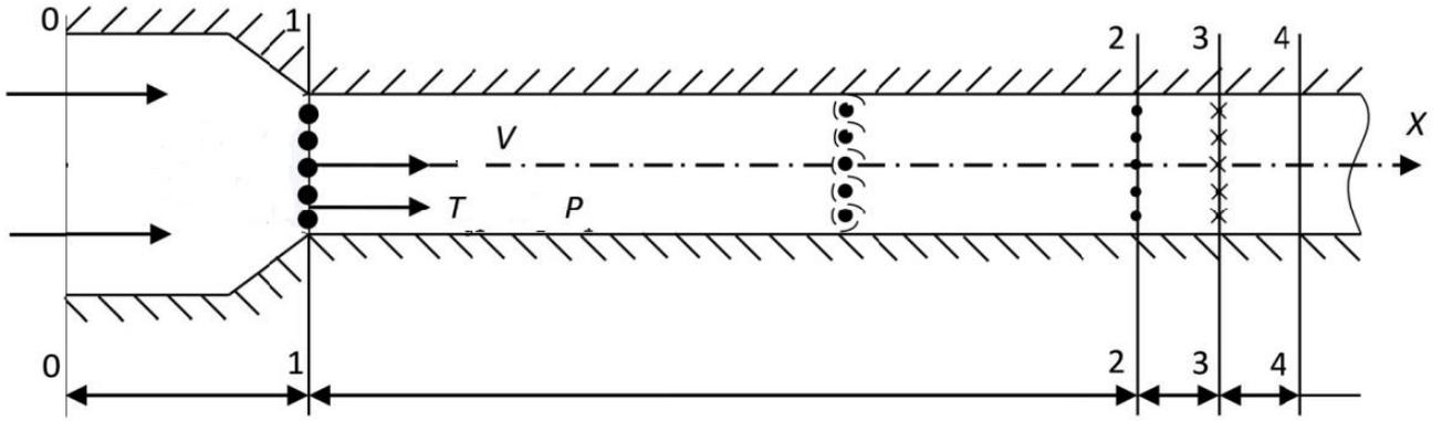
Figure 2- System of the reactor for dispersed combustible aqueous organic composition for treatment using plasma [1].
