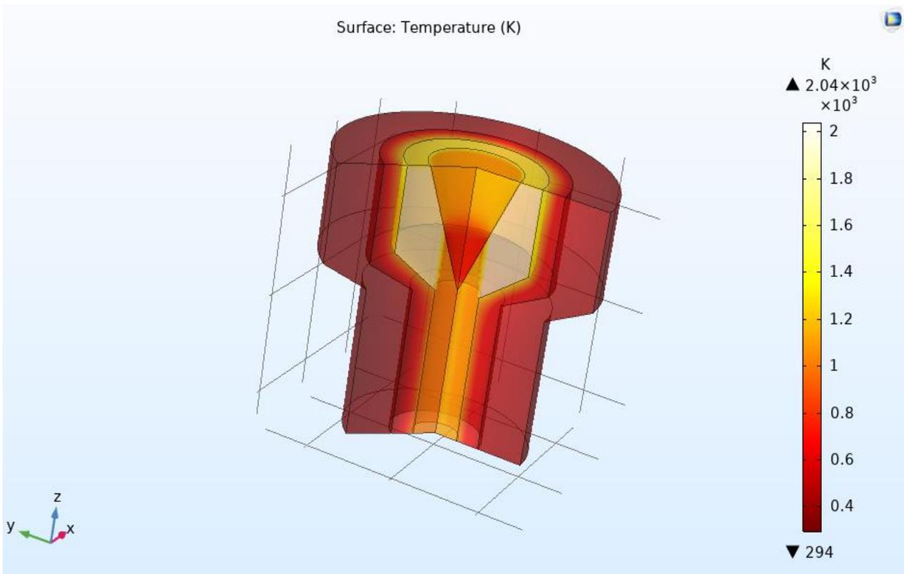
Figure 8- Surface Temperature 3D Distribution for DC Thermal Plasma Plant.
