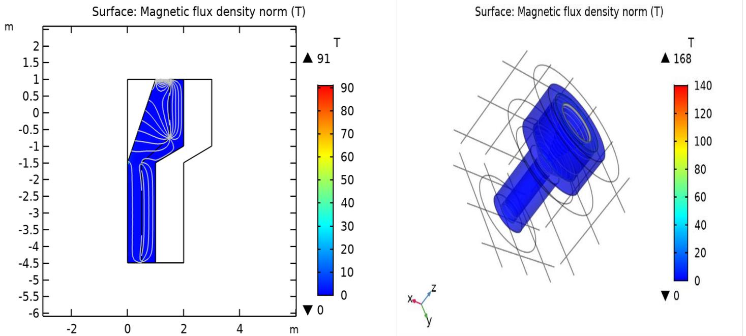
Figure 5- Magnetic flux density distribution.
