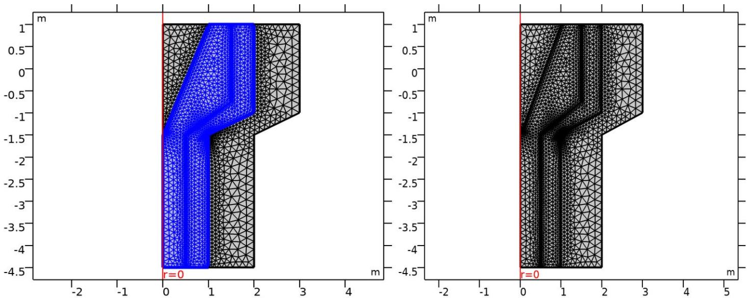
Figure 4 - DC thermal Plasma Plant Mesh, and 2D Plan Mesh with specific domains for Arc plasma flow and Uranyl Nitrate solution.
