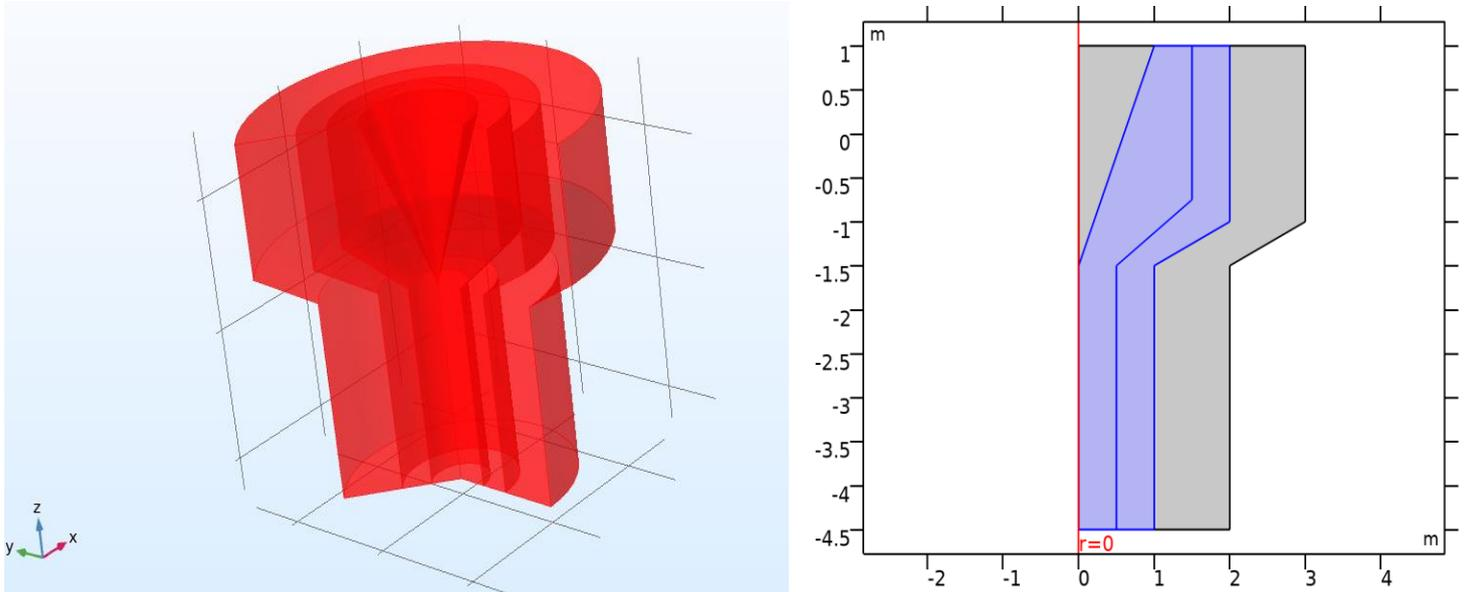
Figure 3- DC thermal with specific domains for Arc plasma flow and Uranyl Nitrate solution. Plasma Plant 3D Distribution, and 2D Plan [6].
