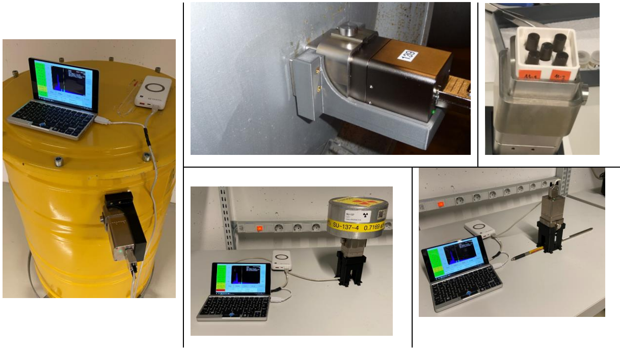
Figure 1. MCCM system in various measurement configurations: container/cylinder (left and top center), bulk material (bottom center), pellets (top right), fuel rod (bottom right).
