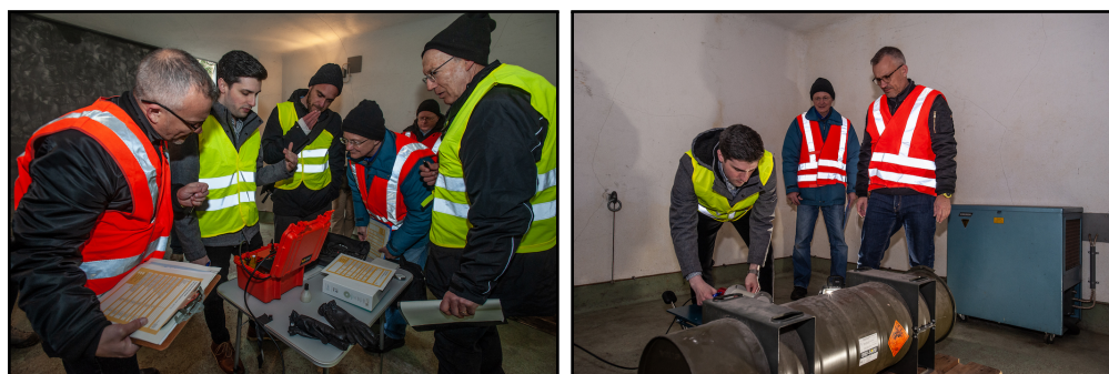
Figure 3: Participants of the Menzingen Inspection Experiment. Left: Host (yellow vests) and inspector (orange vests) teams discussing the operation of the Absence Confirmation Experimental (ACX 2.0) device. Right: Participants set up the sodium iodide detector for passive gamma ray and transmission measurements of the inspected container. Source: Pavel Podvig.
