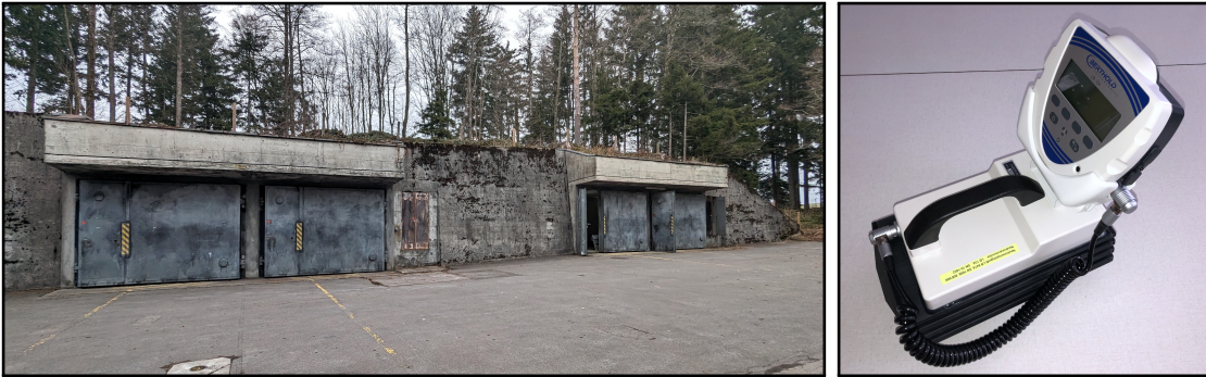
Figure 2: View of the four bunkers used for the radiation measurements (left). The detector used for the neutron measurements (Berthold LB 6414) uses a polyethylene-moderated helium-3 tube and is optimized for plutonium search applications (right). Source: Pavel Podvig and Spiez Laboratory.
