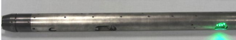
Figure 3. The Graphite Sampling Tool. The forward view camera, on the left, looks down the channel. The umbilical connects to the top of the tool above the sideview camera, which has green LEDs lit. The cutter extends from the hole that is approximately halfway between the forward and sideview cameras.
