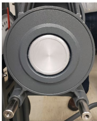
Figure 2: The Aegis™ RDC installed in the ISOCS™ Shield with the collimator removed.
