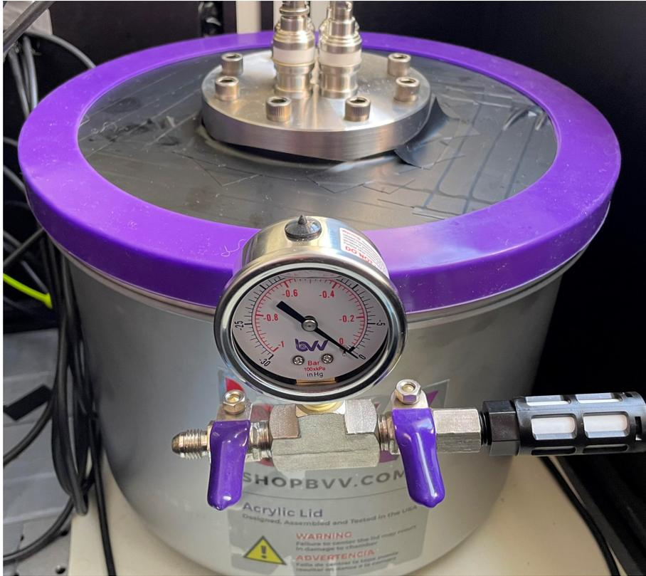
Figure 1: Vacuum chamber used for OCT measurement.
