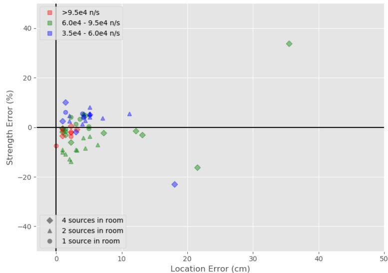
Figure 7. PyMAC's error by source strength and number of simultaneous sources.
