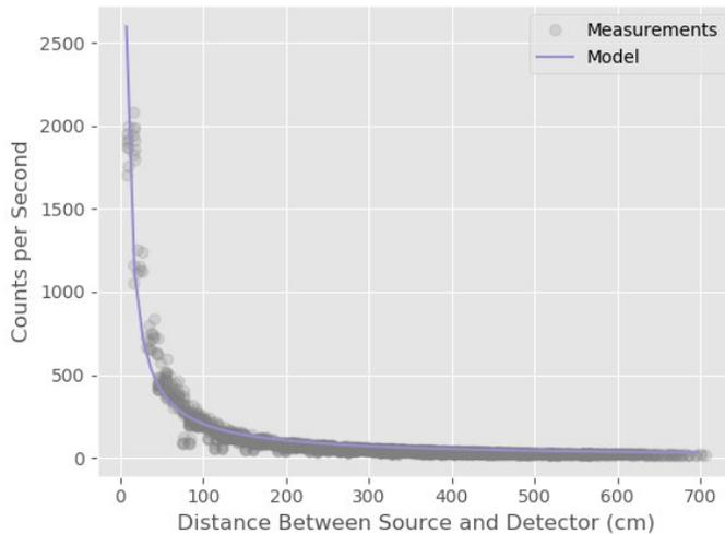
Figure 3. Curve Fit ROM illustrated on top of the data it was fit on.
