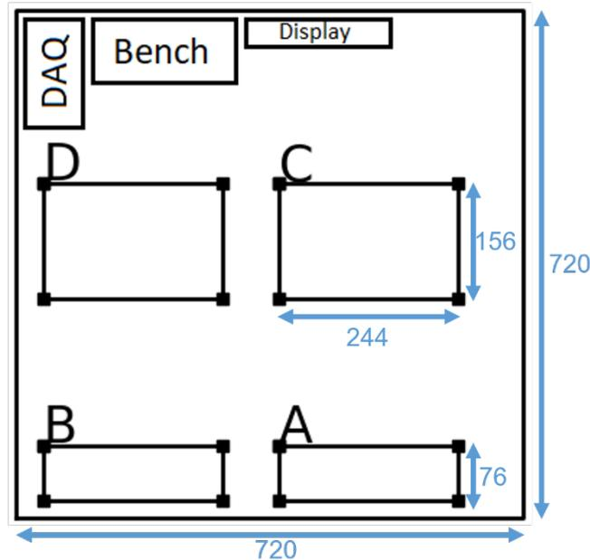
Figure 1. Testbed floorplan illustrating four gloveboxes labeled A, B, C, and D. Squares on the corners of the gloveboxes represent the locations of He-3 neutron detectors.
