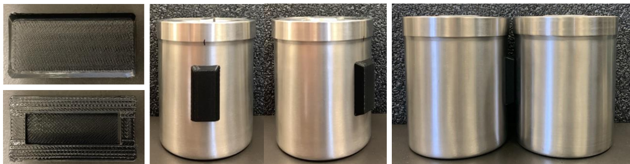
Figure 7. (Left) the additively manufactured prototype container spacer tag cover designed for the Sentry Slim II RFID tag mounted on a 1-quart slip-top container. (Center) the tag cover installed on the container. (Right) an example of the tag cover providing spacing between the tagged container and a neighboring container.
