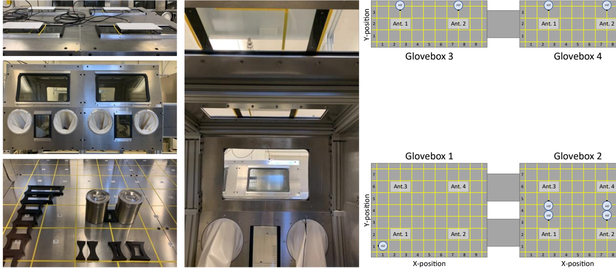
Figure 3. (Top left) The top of Glovebox 1 showing the p12 RFID antennas mounted on the top windows. (Middle left) The front of Glovebox 1. (Bottom left) The Glovebox 1 interior during the Scenario 2 testing, with the targeted tagged container in position 4,3 (x,y). (Middle) The interior of Glovebox 1 showing the location of the p12 antenna mounted above. (Right) A cartoon showing a top-down scale view of Gloveboxes 1-4 along with the positions of the 1-quart containers placed in each glovebox. In all testing, the antennas in Glovebox 1 were powered and the container in Glovebox 1 was the targeted container.
