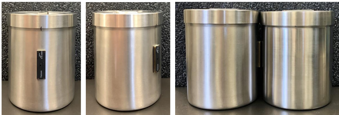
Figure 2. An example of the Sentry Slim II on-metal hard RFID tag mounted vertically on a 1-quart container. The left and center photos show the bare tag, while the right photo shows the tagged container on the left with another container in contact.
