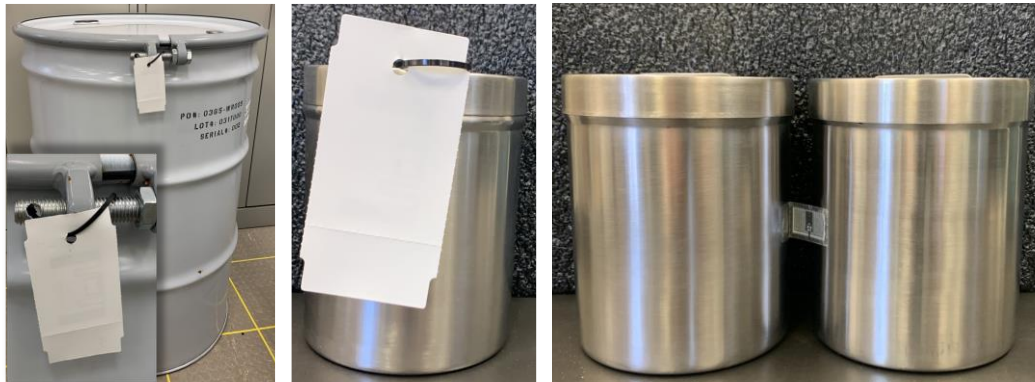
Figure 1. (Left) An RFID hang tag mounted on a 55-gallon drum and (center) a 1-quart slip top container. (Right) An RFID butterfly-style flag tag mounted on a 1-quart slip top container with a second container touching the flag portion of the tag.
