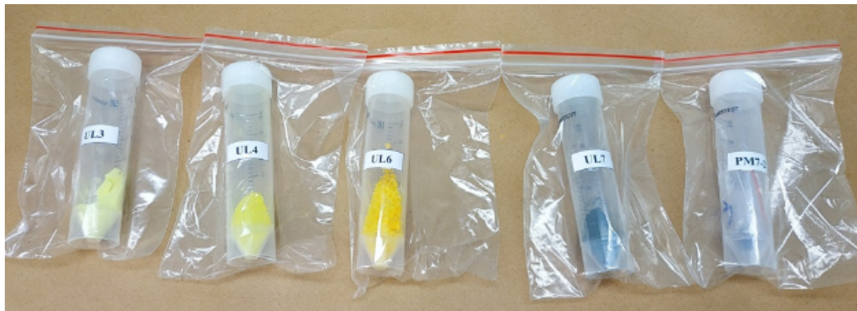
Figure 1: Four uranium powder samples (UL3, UL4, UL6, UL7) and one low-enriched uranium fuel pellet (PM7-2) being analyzed by LLNL and LANL in this exercise. The INP analyzed an equal portion of the same powder samples and a similar pellet (PM7-1).
