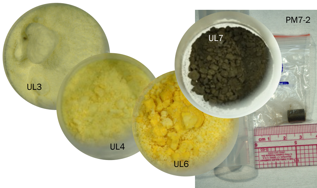
Figure 3: Close-up images of the four uranium powder samples (UL3, UL4, UL6, UL7) and fuel pellet sample (PM7-2) received at LLNL.
