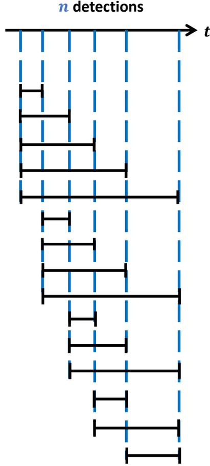
**Figure 1.** A schematic based on [2] detailing the “Type 1” neutron time difference method. In this work it is interpreted as any-and-all forward neutron detection time differences.
