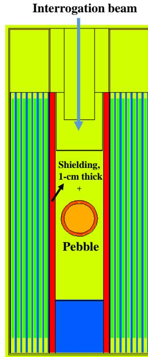
Figure 6: Active interrogation measurement setup.
