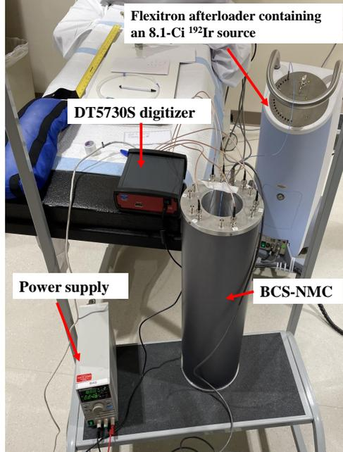
Figure 2: Measurement of the 8.1 Ci  $^{192}\text{Ir}$  HDR source. The gamma-ray source was placed at the center of sample cavity of the NMC and the measurement lasted for 10 min.
