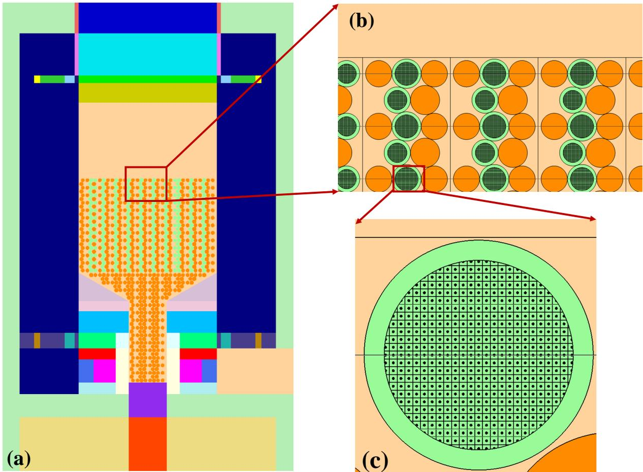
Figure 4: Full SCALE model of HTR-10. (a): Vertical cross-section of the reactor. Green spheres represent the TRISO-fueled pebble and the orange spheres represent the pure graphite pebbles. (b): Zoomed-in view of the mixed pebble region. (c): Zoomed-in view of a single TRISO-fueled pebble, with each black dot representing one TRISO fuel particle.
