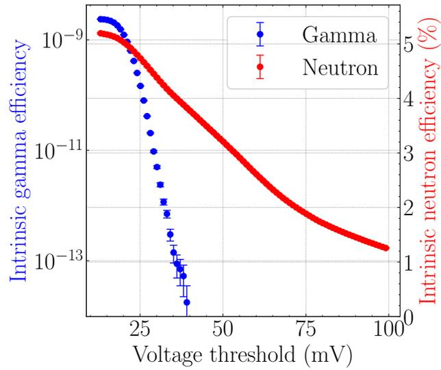
Figure 3: Intrinsic gamma-ray and neutron efficiency as a function of discriminator threshold.
