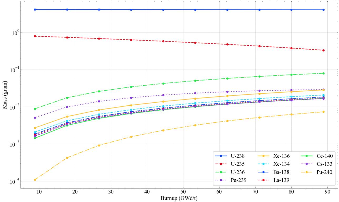
Figure 5: Mass of 10 nuclides of the highest weight fraction as a function of fuel burnup.
