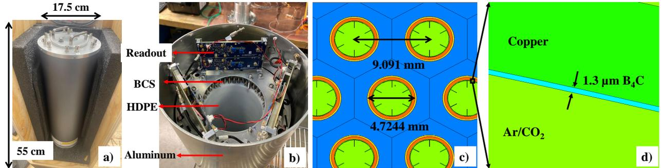
Figure 1: Design of a custom BCS-based NMC for interrogation of TRISO-fueled pebbles. (a) is the external view of the counter, (b) is the internal view with the readout electronics, straws and HDPE, (c) is the cross section of pie-6 straws, and (d) shows the  $1.3 \mu\text{m}$ -thick layer of  $\text{B}_4\text{C}$  converter.
