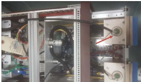
Figure 4. Alpha Duo electronics connected with external detectors, with connector cable soldered on the “green insulator”
