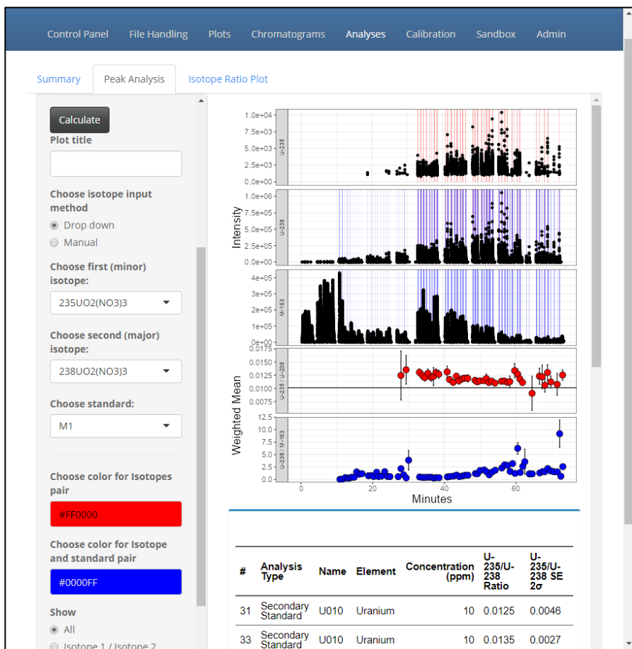
Figure 5. Peak Analysis sub-tab, showing an example of peak-finding logic applied to automatically identify discrete analytical aliquots within a continuous, multi-modal time-series in a single CDF data file.
