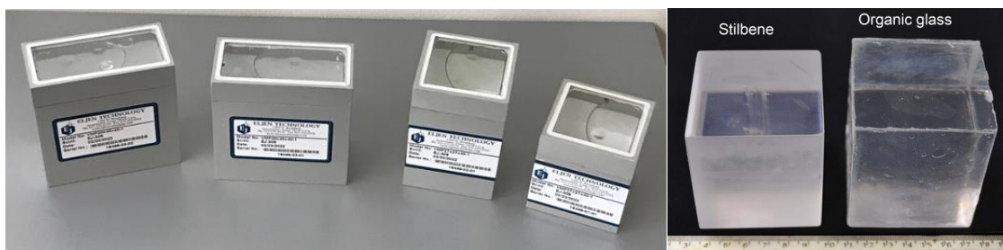
Figure 1. Examples of newly fabricated fast neutron scintillator cells for the optimized detector array investigations: EJ-309 liquid scintillator (various dimensions), Stilbene, OGS cells in smaller volumes (~250ml) for the high cell segmentation design concept.
