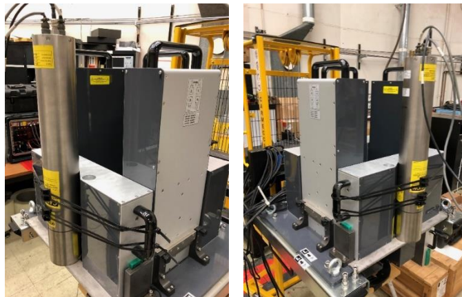
Figure 7. Experimental setup for the Thermo Scientific DD generator coupling with the FNCL instrument using the reverse orientation of the VVER-1000 front shield block.
