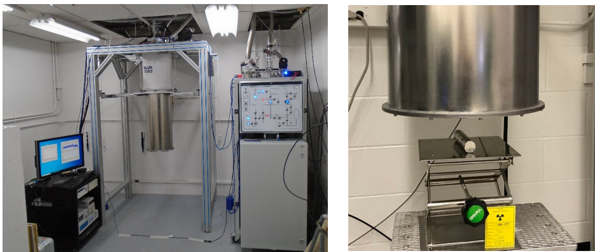
Figure 1: (Left) The INL gamma spectrometer, HERMES-400, in the basement of the INL MFC Analytical Laboratory. The cryostat is the suspended cylinder in the center with its lower half surrounded by a magnetic shield. To the right is the gas handling unit with pumps and valves for the helium gas mixture. To the left is a small electronics rack for data acquisition. (Right) The detector modules face downward, so sources are placed beneath the detector for measurement.
